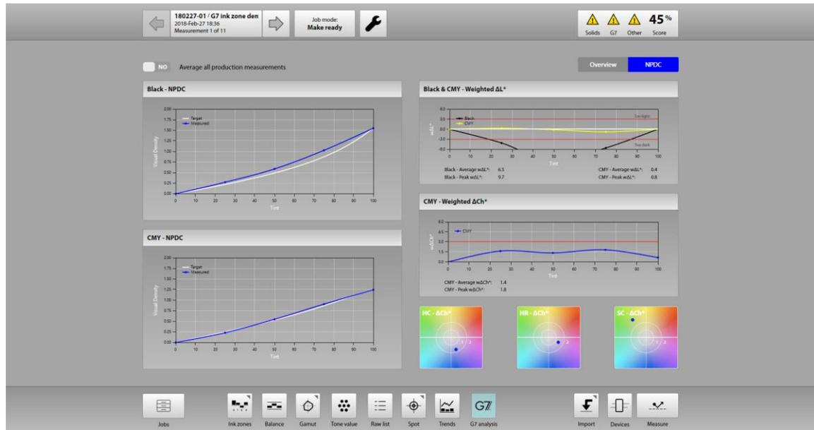
The NPDC tab displays the actual G7 NPDC (target and measured) for K and CMY and also includes the graphs for weighted delta-L and weighted delta-Ch. It also shows average and peak deviations based on the job's tolerance set.
