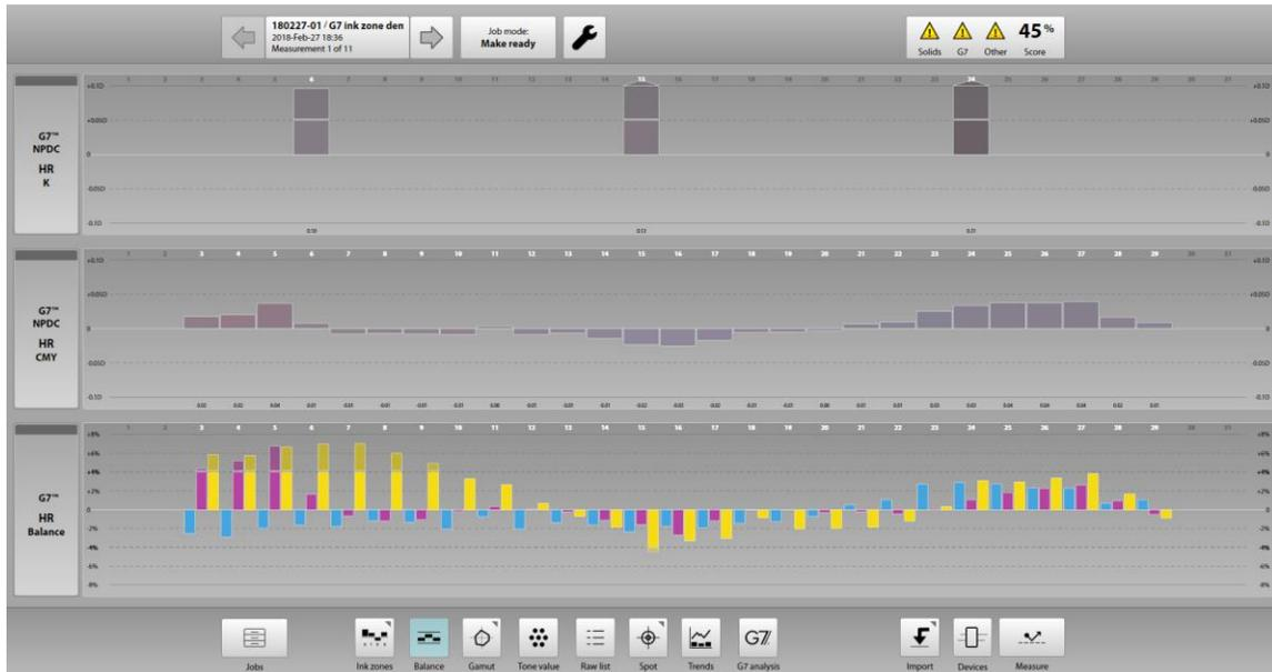
When an ink zone color bar is used, the operator can analyze Gray Balance (HR) and tonality (HR) for CMY and K at a glance. The top two bar graphs clearly show the tonality of the HR patches measured (too high, too low). Please note that the graphs are calculated dynamically based on the actual G7 NPDC target for this measurement.
